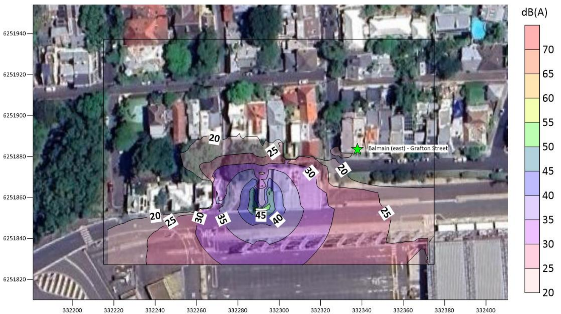
Figure B-2: Predicted night time noise contours (dB(A)) under stability class D for operational activities as designed – Grafton Street close up (including 5 dB penalty for potential tonal characteristics)
