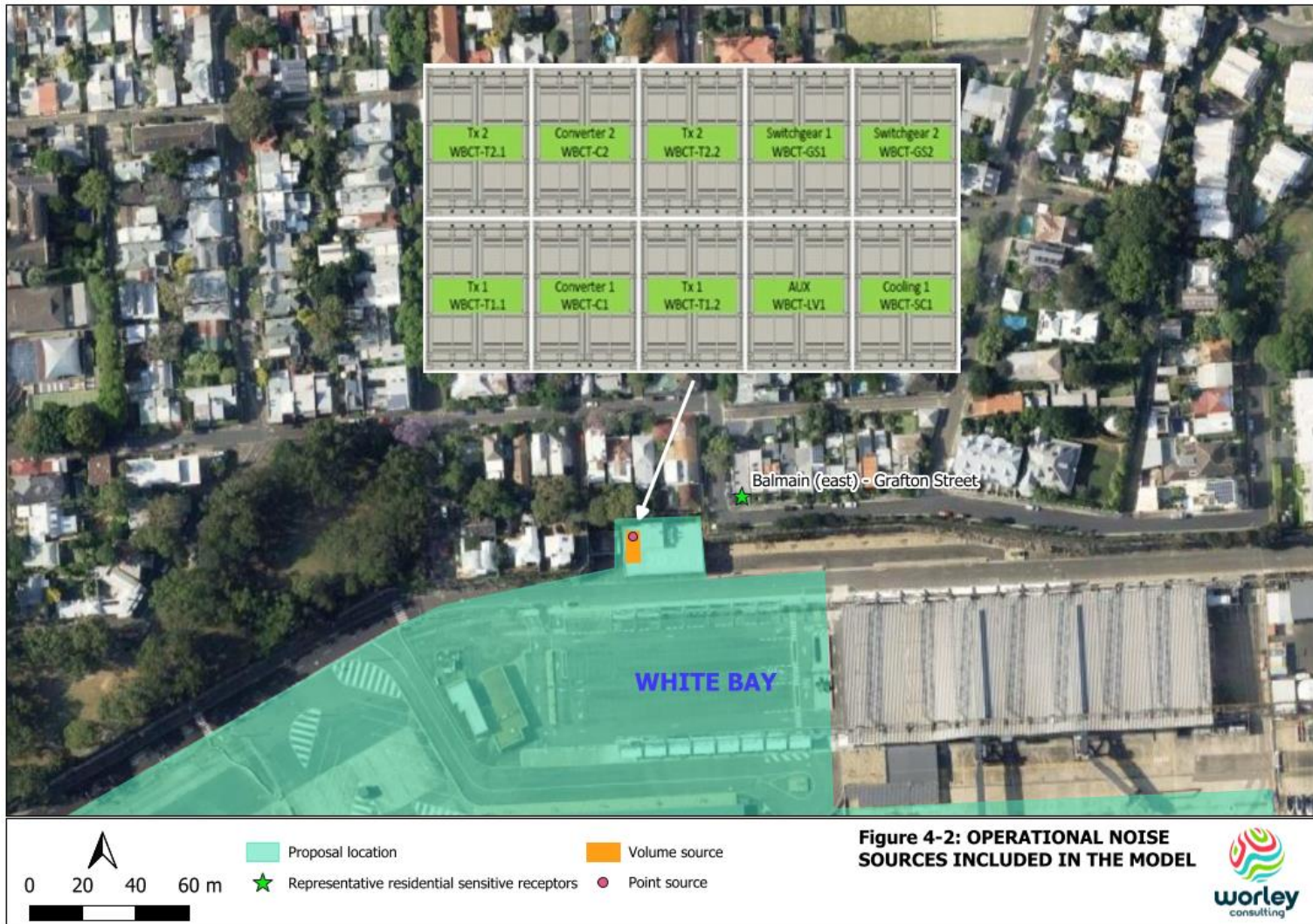
Figure 4-2: Operational noise sources included in the model
