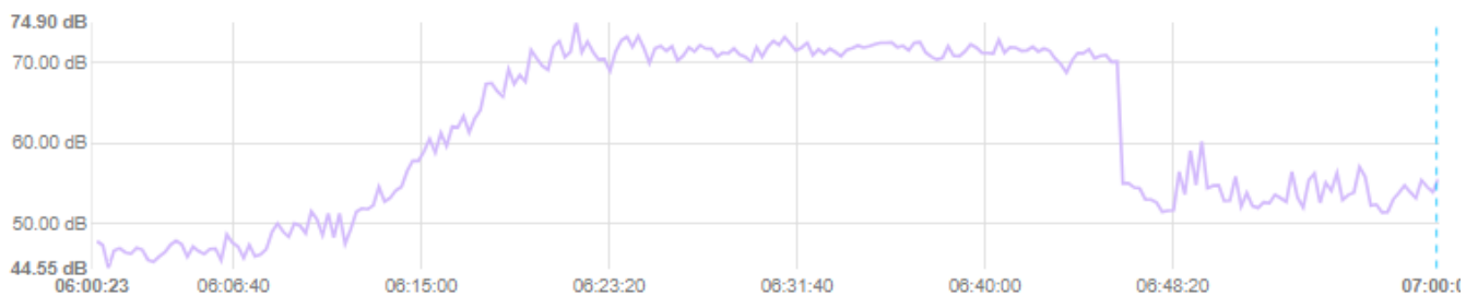
Figure 4.11 A-weighted noise level at L01 as Pacific Adventure entered the WBCT berth
