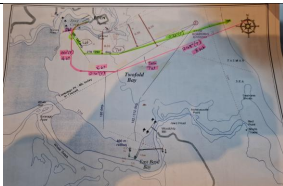
Passage plan for cruise ship showing maximum speeds within the bay area (8 knots in outer area through to 4 knots near the cruise wharf (limit of 10 knots)
