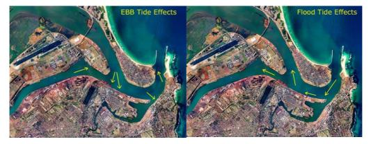
Current rates after heavy rain events can exceed 3-4 kts particularly on an ebb tide.
