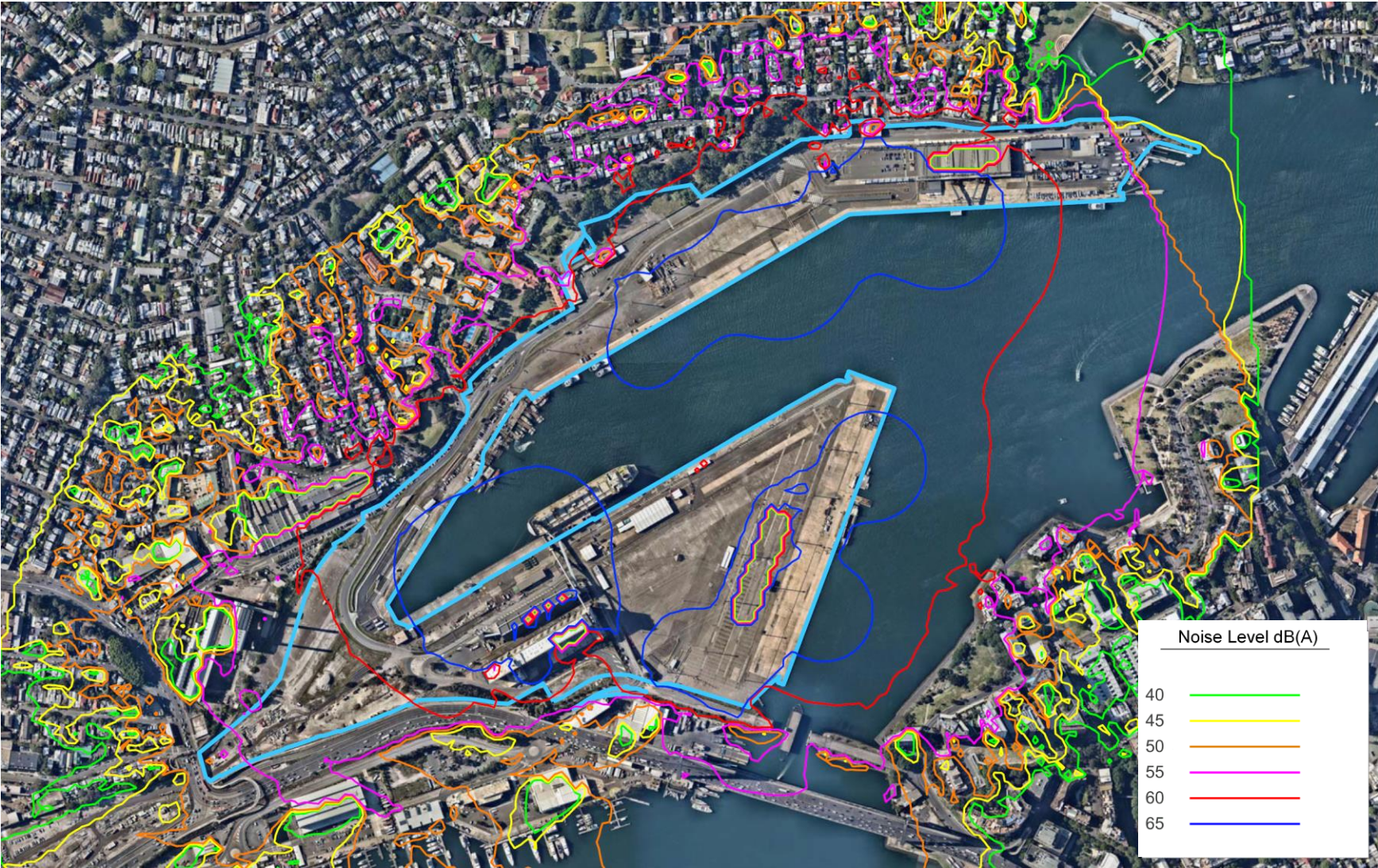
Figure 15: Vessel and landside representative worst case noise level – Daytime (evening is included) 10 years into future
