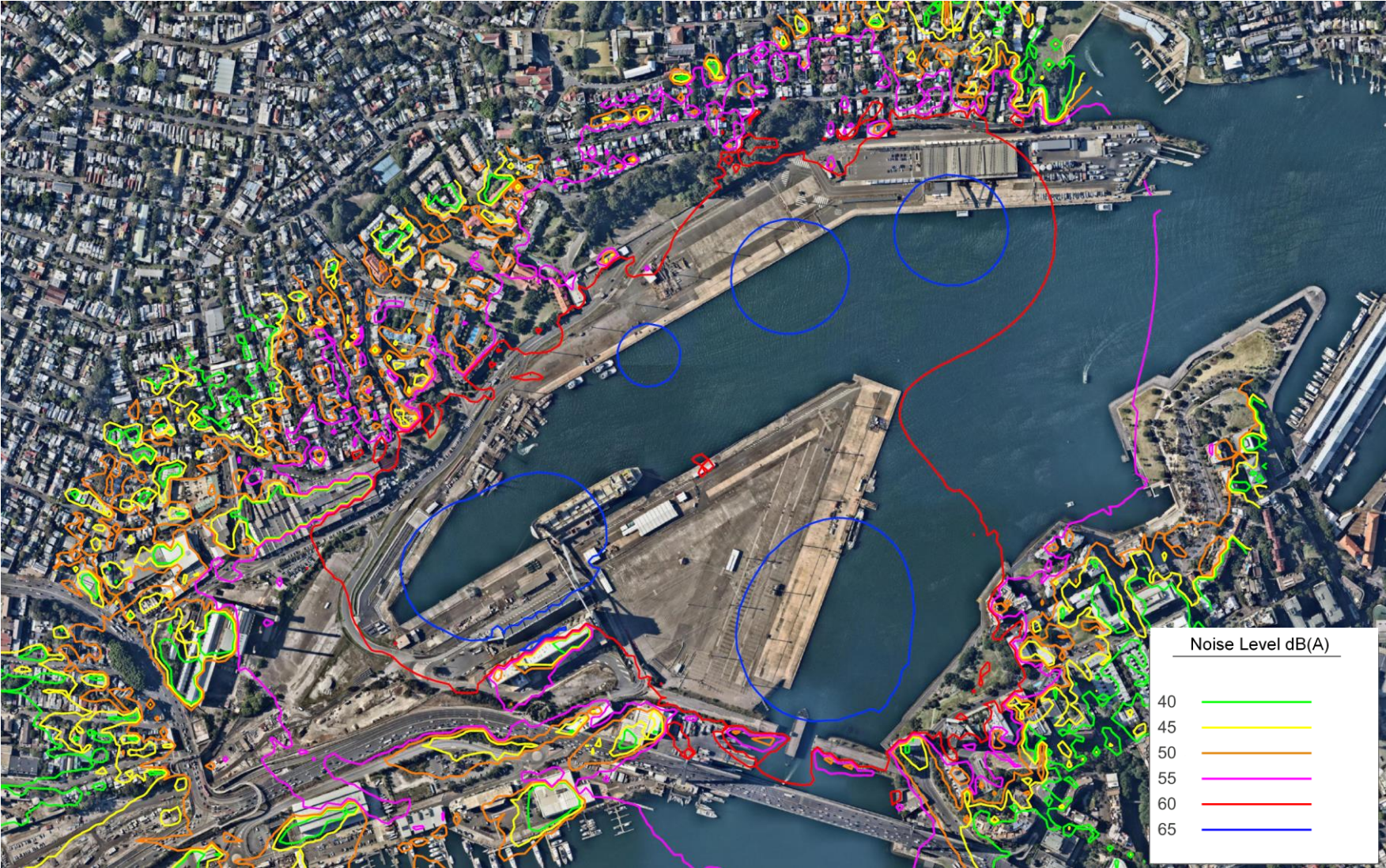
Figure 14: Vessel representative worst case noise level - Daytime (evening is included) 10 years in future
