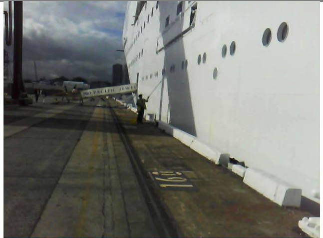
Photo 2 Cleaning of ship hull using water and roller in accordance with painting and washing permit. No detergents or cleaning chemicals are permitted to be used.
